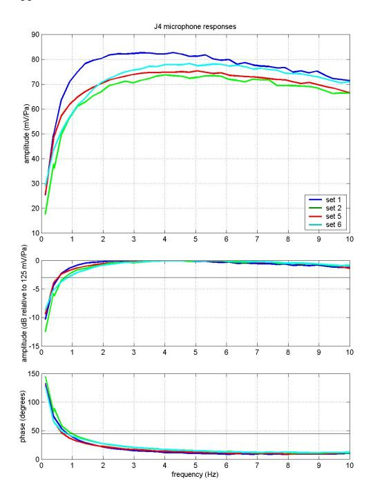
Absolute noise floors for these microphones are difficult to assess in the lab but with the final circuitry configuration, they appear at LEAST as low as 3 mV (or about 0.04 Pa). However the lab is a noisy environment and we should expect better in the field (at least when wind noise is low). Note that the benefit of using four microphone elements in each instrument is to improve the inherent noise floor in the near-infrasound bandwidth.
